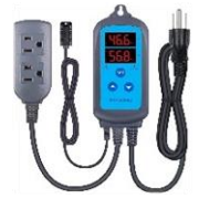
Hygrometer that regulates power to a humidifier
